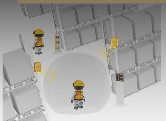
Through the installation of a virtual gateway, it is possible to carry out a HandFree access control and people counter without the need for physical barriers.
